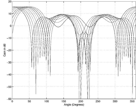
Figure 5: Ten antenna patterns between 0° and 60° at 6° steps.
