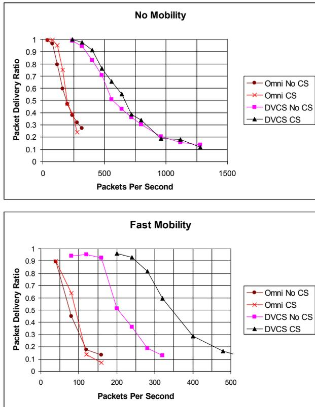
Figure 9: PDRs with and without the physical CS.
