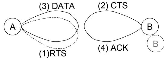
**Figure 1: Negotiation between the source and the destination.**
