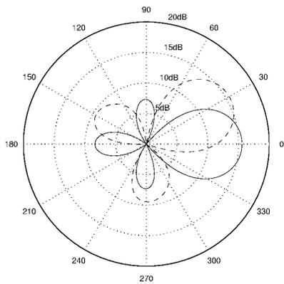
Figure 4: Two antenna patterns bearing 0° and 30°.
