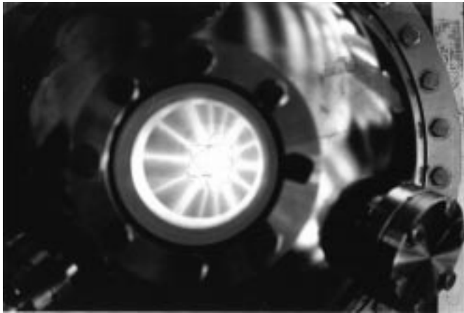
Fig. 4. Digital photograph of the Star mode, taken through the IEC viewport. The microchannels and dense “core” plasma are clearly visible.
