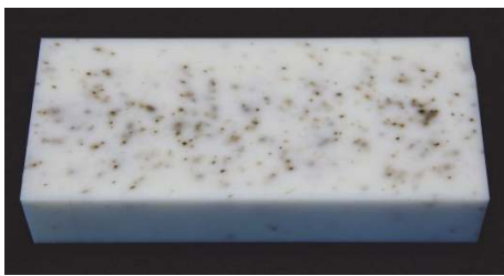
FIGURE 8: A block (200 mm × 80 mm × 40 mm) of HMW-PE with black spots that appeared after 31 days of pure thermal aging at 125°C.
