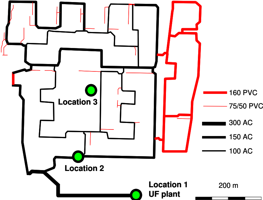
Fig 3-2 Research Area supplied with UF water. The red lines represent PVC pipes, the red lines AC pipes. Diameter indications for PVC pipes are typical outside diameters and AC typical inside diameters. Location 1, 2 and 3 are the particle count monitoring locations
