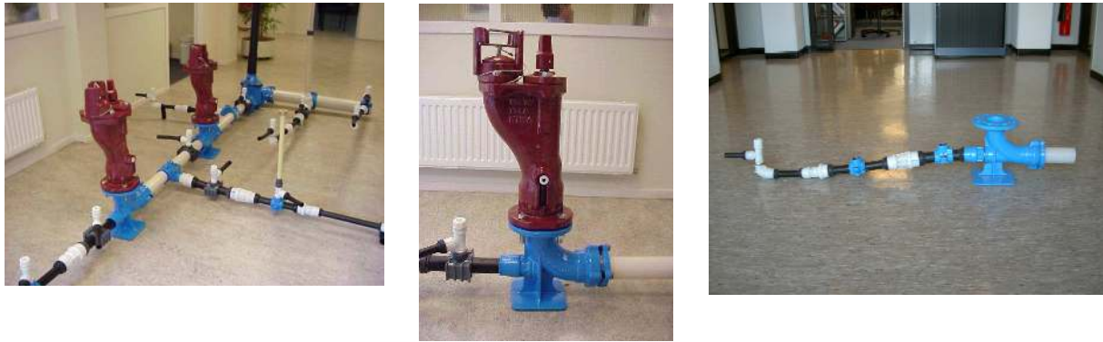
Fig 4-7 Example of technical layout of new network and newly designed 30 m 3 /h fire hydrant
