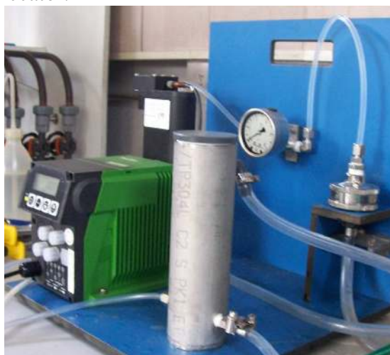
Fig 2-20 TILVS-unit. On the left is the pump, in the middle the water overflow vessel and on the right the filter unit.
