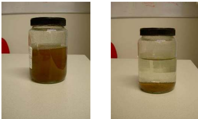
Fig 2-1 Samples handed in by customers. Left the discolouration incident and right the sample after settling
