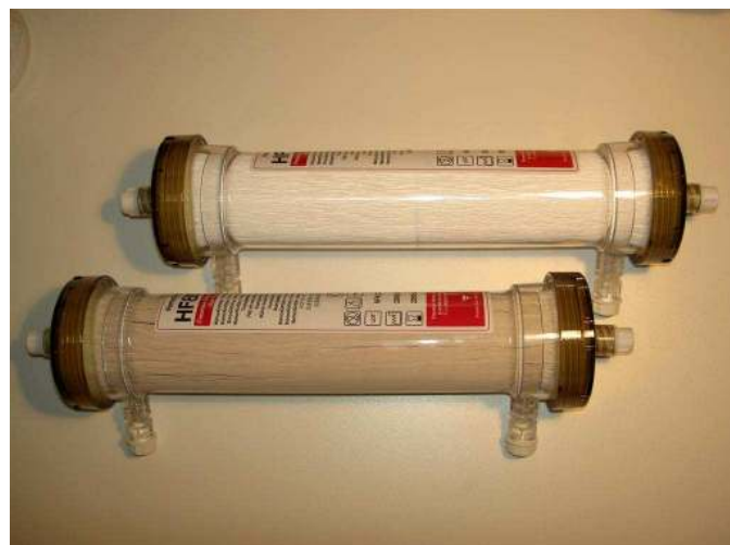
Fig 3-23 Picture of Hemoflow filters pre- and post-sampling. The increased colour suggests that some of the particles are left in the filter, thus clouding the accuracy of the sample
