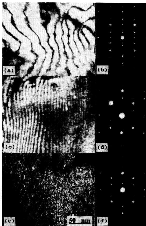
FIG. 3. Dark-field images (type X ) and the corresponding diffraction patterns from three widely separated regions showing the variation of DC line spacing from about 20 to 6 to 2 nm.
