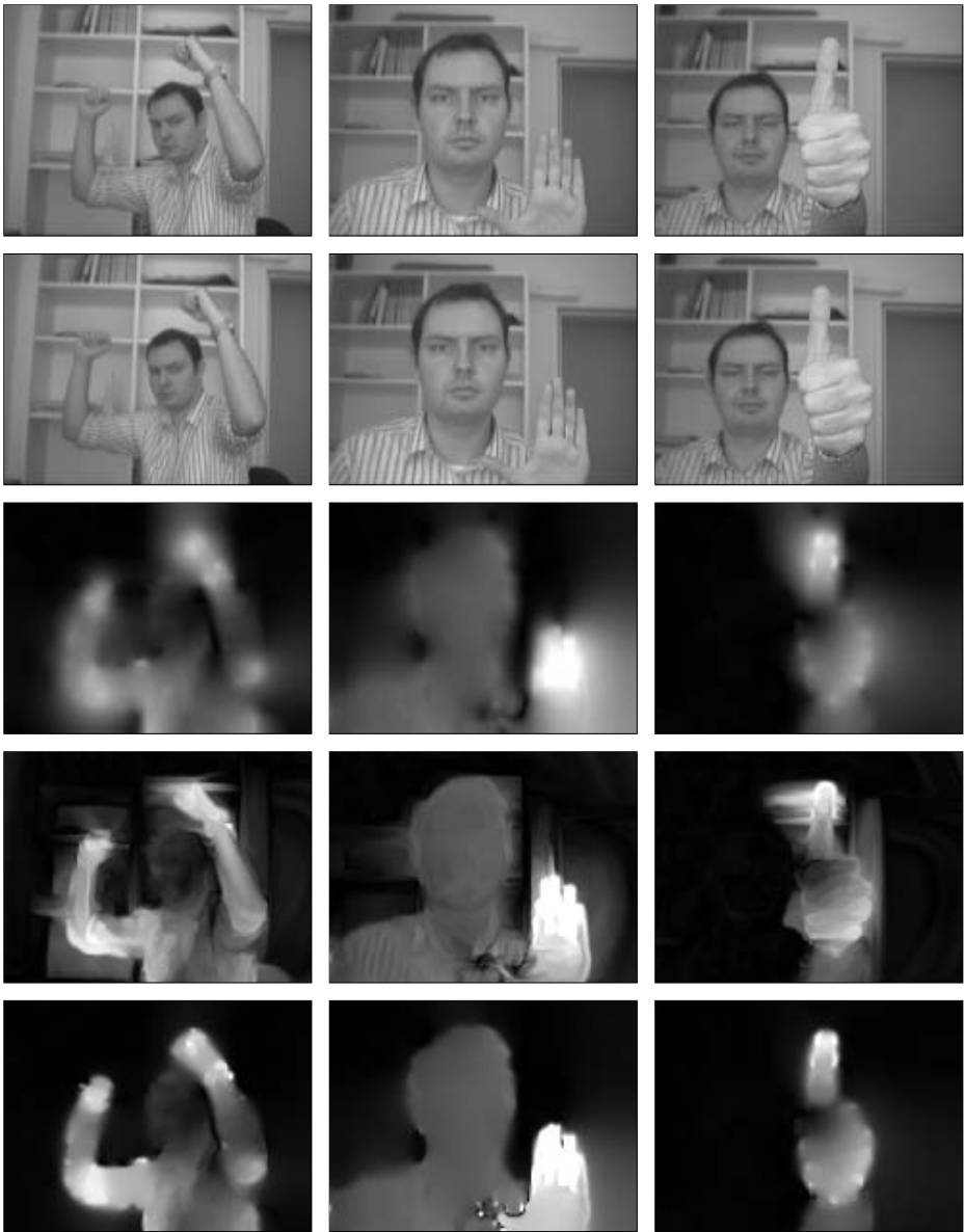
Fig. 1. Left to right: dancing sequence, waving sequence, rotating thumb sequence. Top to bottom: first frame, second frame, our CLG multigrid implementation from [8], our Nagel-Enkelmann multigrid implementation, our TV-based regularisation FAS multigrid implementation. Brightness code: The magnitude of a flow vector is encoded by its brightness. Brighter pixels stand for larger displacements. Color versions of the flow fields are available at http://www.mia.uni-saarland.de/bruhn/scsp05/flowfields/
