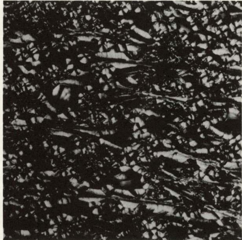
Figure 27. PULP MOLDED AND CARBON VAPOR INFILTRATED TO A DENSITY OF 1.6 gms/cc. (250X)
