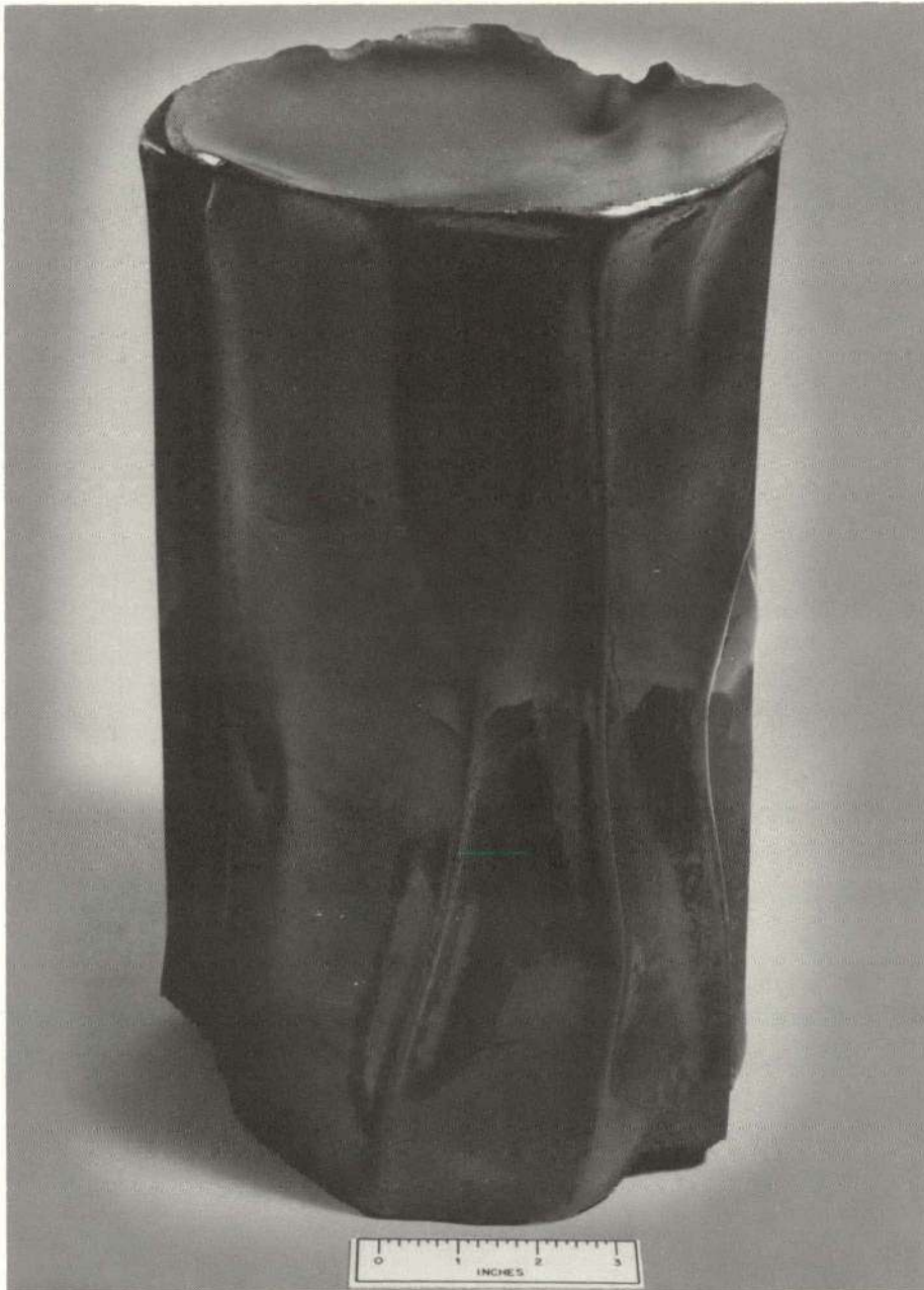
Figure 5. PRESSURE-CARBONIZED BILLET OF AN ISOTROPIC CASTING.
