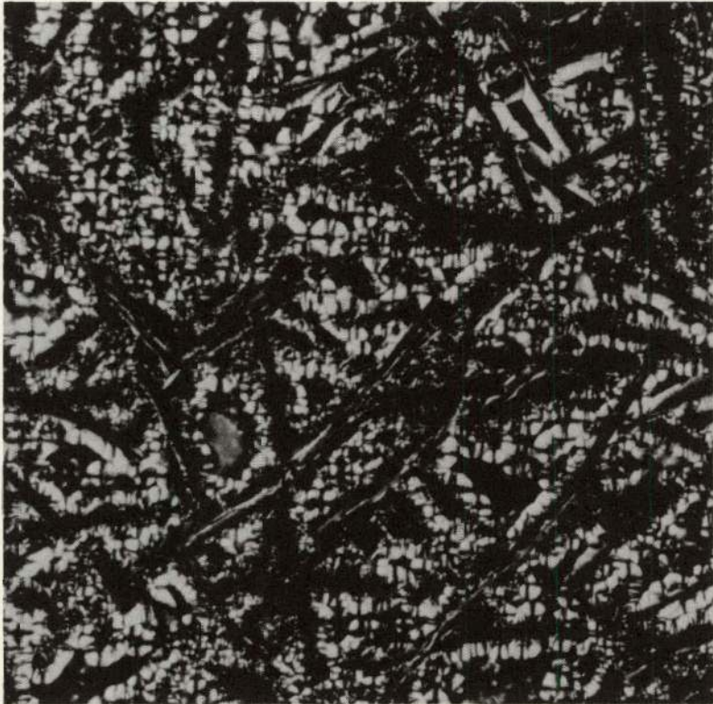
Figure 27. PULP MOLDED AND CARBON VAPOR INFILTRATED TO A DENSITY OF 1.6 gms/cc. (250X)
