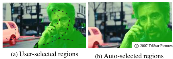
Figure 11: User selects regions in a single frame (a) by roughly brushing over objects of interest (indicated by dashed line). These regions are automatically extrapolated to other frames (b) of the video. See accompanying video. Original frame from 88 minutes, ©2007 TriStar Pictures.
