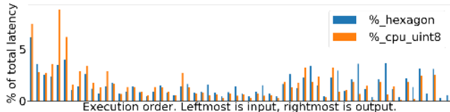
Figure 2: Per layer profiling of MobileNetV3 minimalistic on Pixel4 CPU uint8 and DSP (Hexagon). The leftmost is the input layer while the output layer is on the right.
