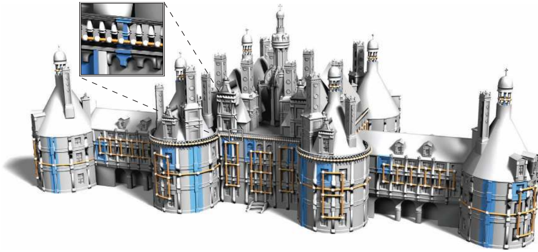
Figure 13: Our method detects multiple 1- and 2-parameter structures. The blue regions denote the representative elements. All structures were detected with 30k samples distributed uniformly across the model, except for the balustrade, for which the rate was increased to 100k.
