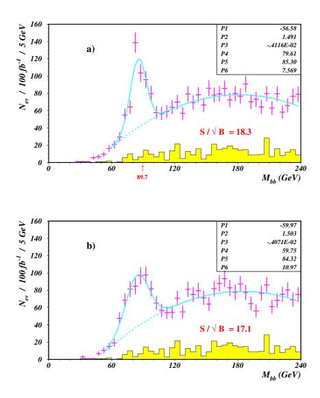
Figure 9.5: Effect of the assumed single hadron energy resolution on the signal visibility: a) the nominal HCAL performance,  $\sigma_E/E = 82\%/\sqrt{E} \oplus 6.5\%$  at  $\eta \sim 0$ ; b) the HCAL energy resolution deteriorated to  $120\%/\sqrt{E} \oplus 10\%$ . mSUGRA point as in Figs. 9.2-9.4.
