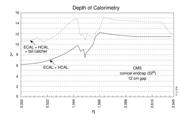
Figure 4.5: Depth of calorimetry and total sampled depth including the tail catcher layers as a function of rapidity in CMS.
