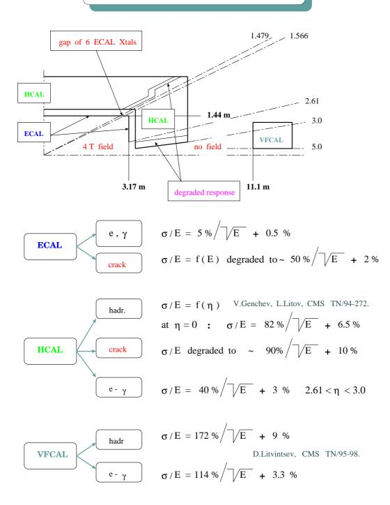
Figure 4.15: The CMS calorimetry model in CMSJET 3.5
