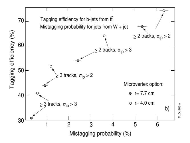
Figure 4.14: Tagging efficiency for b-jets and mistagging probability as a function of the inner barrel pixel layer radius.
