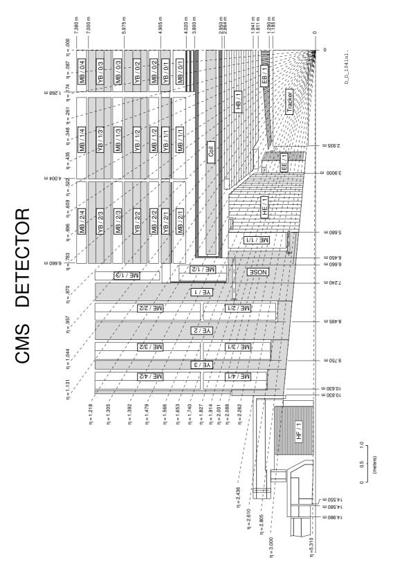
Figure 4.1: Longitudinal cut through the CMS detector. The tower structure of the hadron calorimeter and the arrangement of the electromagnetic calorimeter crystals is indicated, as well as the locations of the tail catcher layers.
