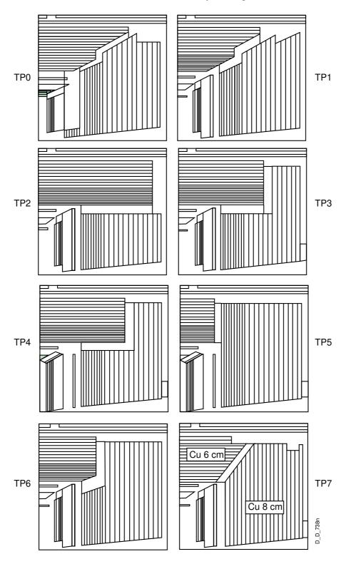
Figure 4.7: Various configurations of the barrel/endcap calorimetry transition region considered.
