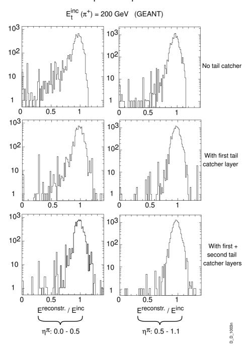
Figure 4.6: Effects on hadron energy measurements of tail catcher layers in the central and next-to-central CMS wheels i.e. in two adjacent rapidity ranges.
