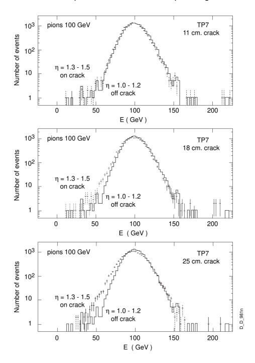
Figure 4.8: Effects on hadron energy measurements of the crack for services between the barrel and the endcap calorimetry for three crack sizes.
