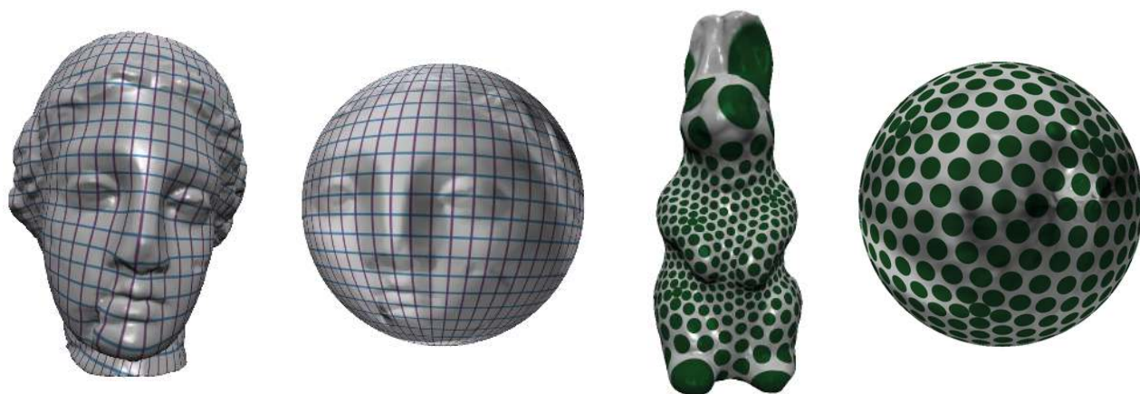
Fig. 7: The Hygeia (50K triangles) and rabbit (26K triangles) models parameterized over the sphere with the parameterization visualized through textures. In the case of Hygeia a grid of latitude/longitude lines. The rabbit is textured with points in an icosahedral pattern. Note the typical area distortion when mapping the head and ear regions to the sphere. No less, the roundness of the texture dots is well preserved through the mapping.
