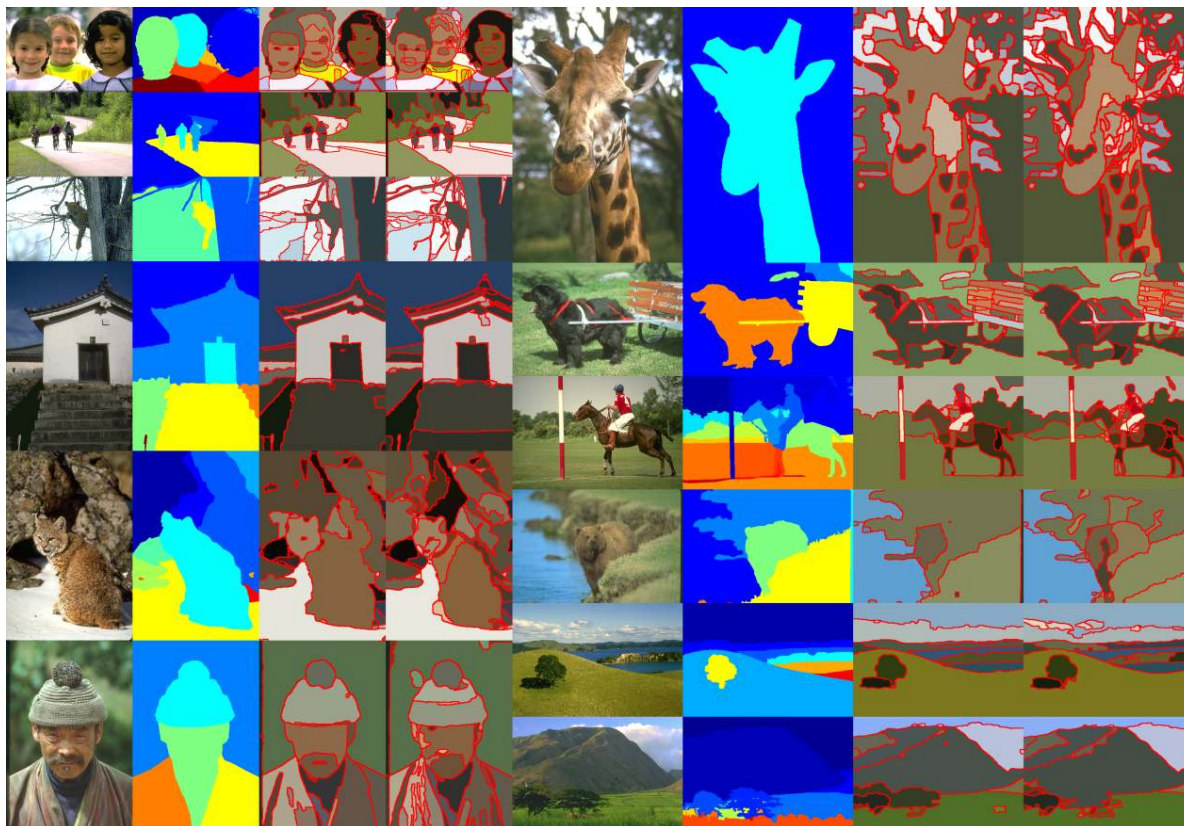
Figure 2: Exemplary segmentation results on Berkeley BSDS 500 obtained on the optimal database scale. First: input image, second: ground truth, third: our result, fourth: UCM result. The obtained segments are mapped to their mean RGB value and boundaries between segments are highlighted, to be able to see if the main image details are preserved.
