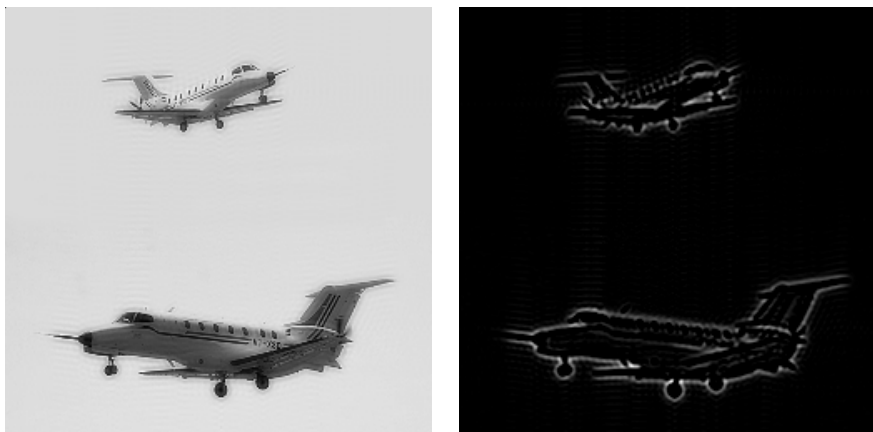
Figure 8. Fused and error image with two levels D=2 of decomposition using MDCT.
