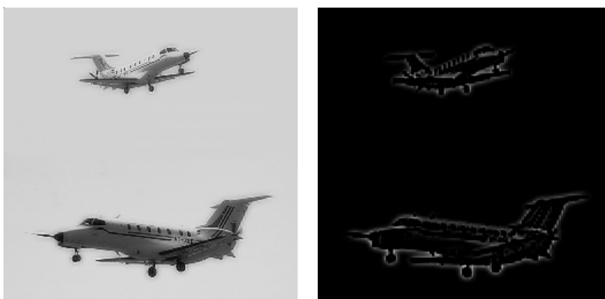
Figure 9. Fused and error image with two levels D=2 of decomposition using wavelets.
