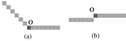
Fig. 1 Examples of a corner model and the local variation of a curve. (a) A corner model, (b) Local variation of a curve.
