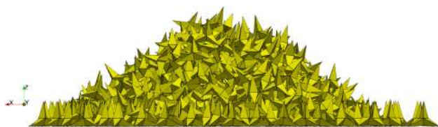
Fig. 28 Lateral view of the final configuration obtained after collapsing the box of tetrapods
