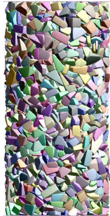
Fig. 4 Image of numerical triaxial specimen, showing potential particle representation of railway ballast
