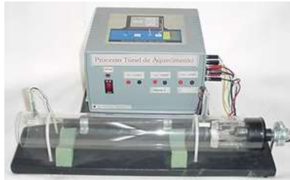
Figure 5. Heating tunnel process used in the practical experiment.
