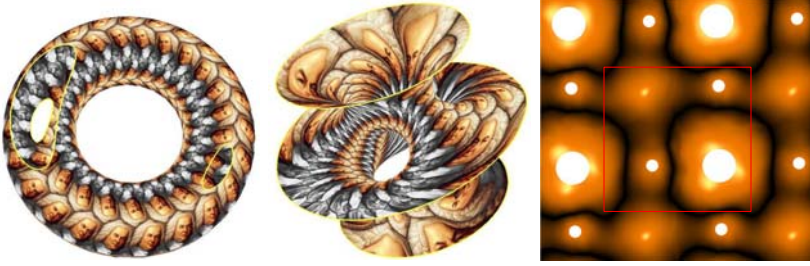
Fig. 12. Two genus one surfaces with 3 boundaries are conformally parameterized onto the plane, such that their boundaries are mapped to circles. Then a map is constructed between their planar images, which induces a matching between them. The matching is visualized by the consistent texture mapping.
