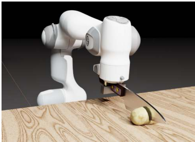
Fig. 1: A rendering from our differentiable cutting simulator. DiSECT provides accurate gradients of the cutting process, allowing us to efficiently fit model parameters to real-world measurements, and optimize cutting motions.
