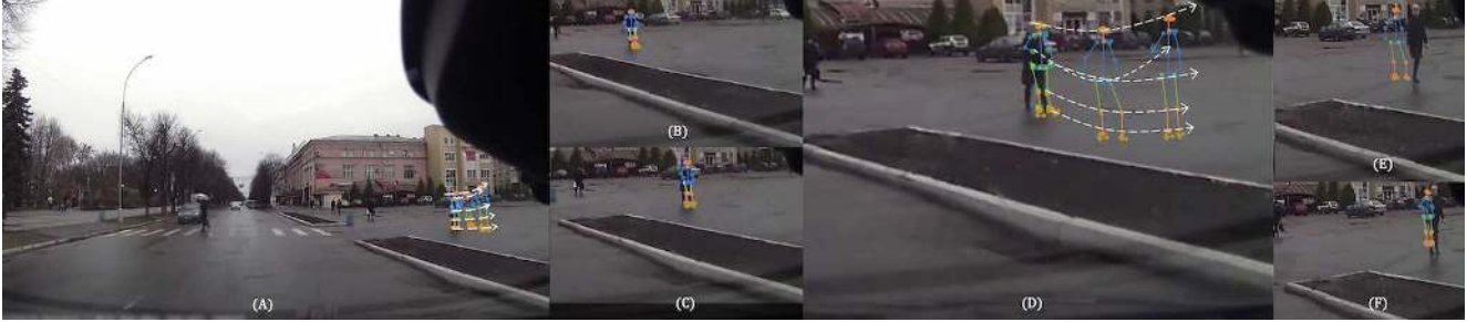
Figure 8: Qualitative pose prediction results. (A) the t_p = 15 length input sequence of poses. (B) and (C) the cropped frames with the pedestrian and the corresponding filled in pose at the start and end of the input sequence. (D) the prediction pedestrian locomotion for the next t_f = 15 frames. (D), (E), and (F) the predicted poses at the start, intermediate, and end of the output sequence, respectively. Video visualizations are available at: https://karttikeya.github.io/publication/plf
