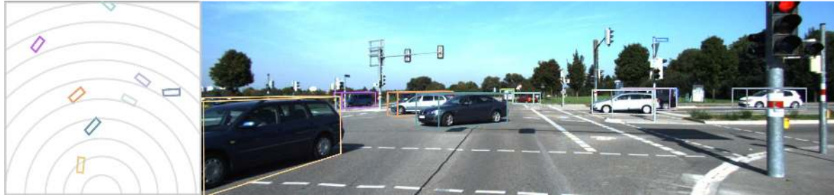
Figure 1: Results obtained from our single image, monocular 3D object detection network MonoDIS on a KITTI3D test image with corresponding birds-eye view, showing its ability to estimate size and orientation of objects at different scales.
