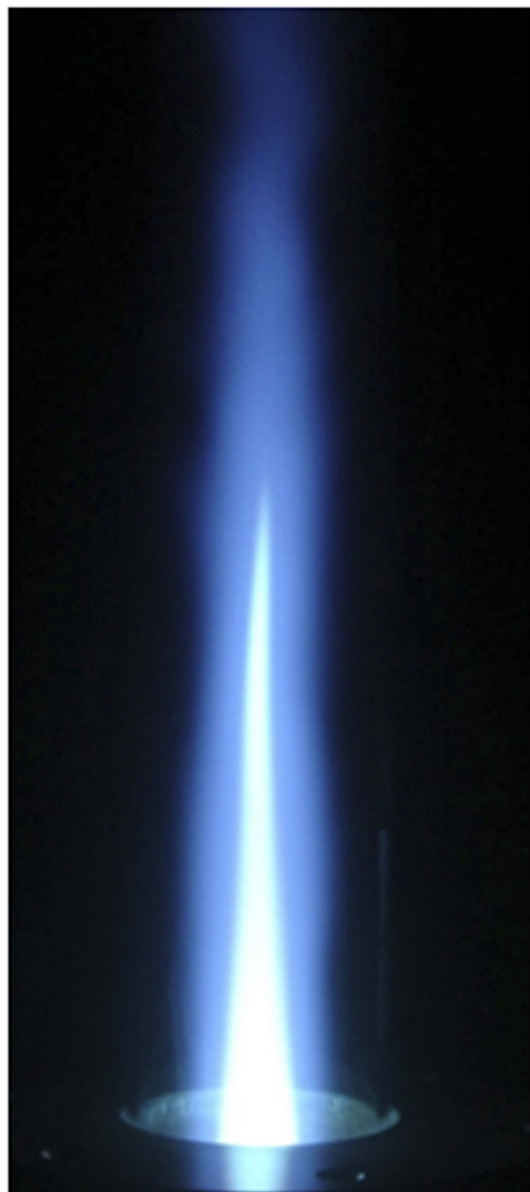
Figure 7. The flame of carbon dioxide plasma torch. Typical carbon dioxide torch shows inside a quartz tube with a 3 cm diameter and a length of 30 cm. The torch is powered by 2 kW of microwave power. The torch volume is almost linearly proportional to the microwave power. The carbon dioxide torch exhibits two distinctive regions: a bright, whitish region of a high-temperature zone and a bluish, dimmer region of a relatively low-temperature zone. The bright, whitish region is a typical torch based on plasma species and the bluish, dimmer region is carbon monoxide recombining with oxygen.
