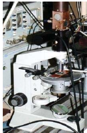
Fig. 2. The experiments with modernised differential-phase scanning laser microscope
