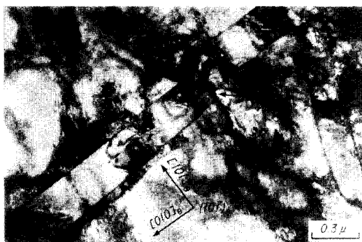
Photo. 12 Plastic deformation of lamellar cementite in 1.25% C steel cold-rolled to 45% reduction after furnace cooling
