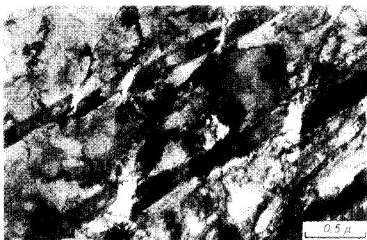
Photo. 13 Fracture of lamellar cementite in 1.25% C steel cold-rolled to 45% reduction after furnace cooling
