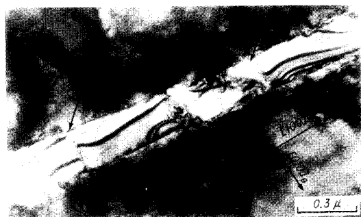
Photo. 11 Plastic deformation of lamellar cementite in 1.25% C steel cold-rolled to 25% reduction after furnace cooling
