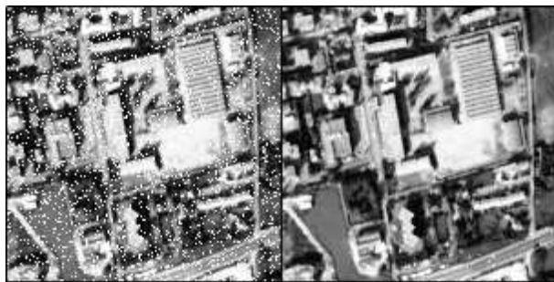
Fig. 5. Left : noisy image (impulse noise, frequency = 10%). Right : occlusion detection is performed by means of the grain filter. Disocclusion is then achieved with our level-lines based algorithm.
