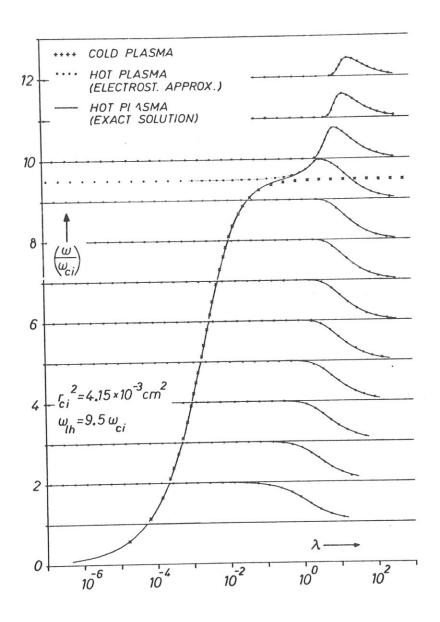
Fig. 8 Comparison of the exact solution of the ion modes with the electrostatic and cold-plasma approximations with  $r_{ci}^2 = 4.15 \times 10^{-3} \text{ cm}^2$  and  $\omega_{\ell h}^2 = 9.5 \omega_{ci}^2$
