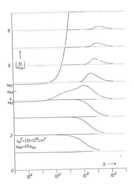
Fig. 2 Generalized electron Bernstein modes with r  $_{\rm ce}^2$  = 1.13 x lo  $^{-6}$  cm  $^2$  and  $\omega_{\rm uh}$  = 4.5  $\omega_{\rm ce}$
