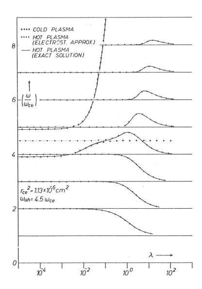
Fig. 5 Comparison of the exact solution of the electron modes with the electrostatic and cold-plasma approximations with  $r_{ce}^{\ 2}=1.13\times 10^{-6}$  and  $\omega_{uh}^{\ 2}=4.5~\omega_{ce}$
