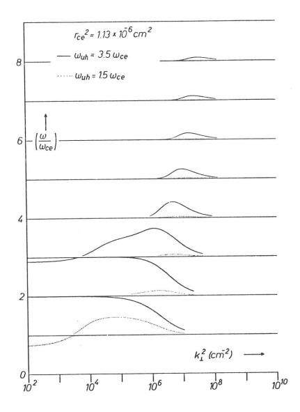
Fig. 4 Generalized electron Bernstein modes with  $r_{ce}^2 = 1.13 \times 10^{-6} \text{ cm}^2$ , and  $\omega_{uh} = 3.5 \omega_{ce}$  (solid curve) and  $\omega_{uh} = 1.5 \omega_{ce}$  (dotted curve)
