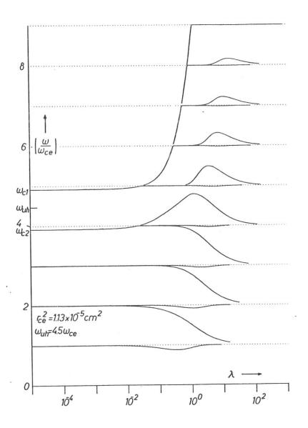
Fig. 3 Generalized electron Bernstein modes with  $r_{ce}^2 = 1.13 \times 10^{-5} \text{ cm}^2$  and  $\omega_{uh}^2 = 4.5 \omega_{ce}^2$
