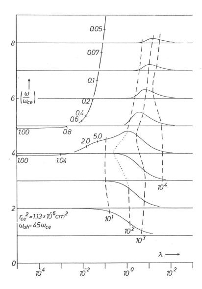
Fig. 7 The polarization of the generalized electron Bernstein modes. The dashed lines (dotted in regions of uncertain computational accuracy) are contours of constant R defined in (26)
