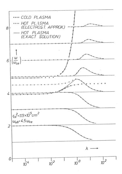
Fig. 6 Comparison of the exact solution of the electron modes with the electrostatic and cold-plasma approximations with  $r_{ce}^{\ 2}=1.13\times 10^{-5}~{\rm cm}^2$  and  $\omega_{uh}^{\ =4.5}~\omega_{ce}$
