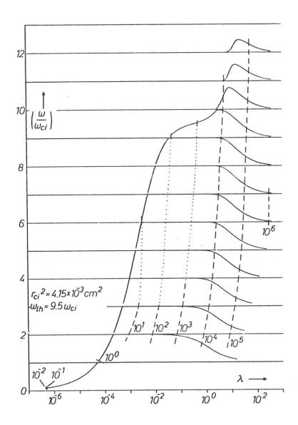
Fig. 1o The polarization of the generalized ion Bernstein modes. The dashed lines (dotted in regions of uncertain computational accuracy) are contours of constant R defined in (26)
