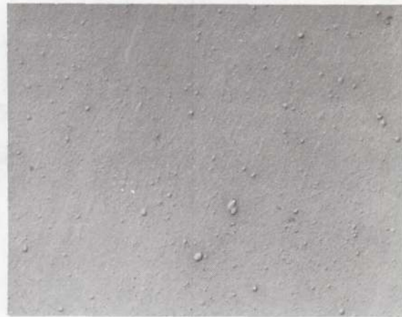
(b) High strength NiO-4ThO 2 (heptane). Twenty-one cold-roll - anneal cycles; ultimate tensile strength, 26 000 psi (182 MN/m 2 ).
