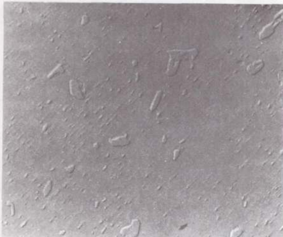
(a) Seven cold-roll - anneal cycles; ultimate tensile strength, 11 500 psi (80 MN/m 2 ).
