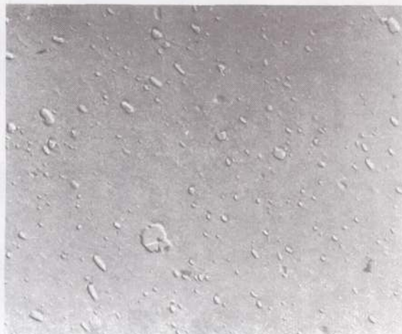
(b) Fourteen cold-roll - anneal cycles; ultimate tensile strength, 14 000 psi (98 MN/m 2 ).
