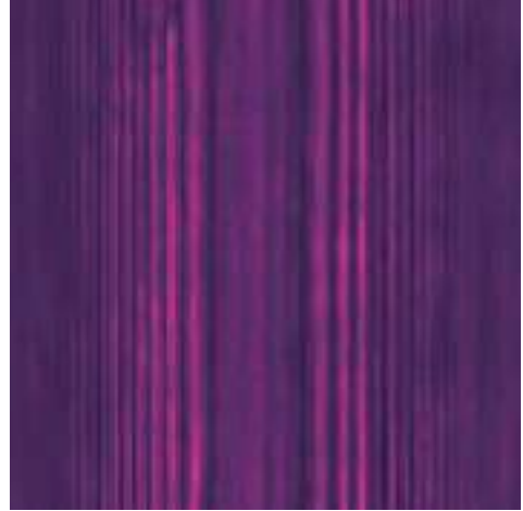
Figure 26: Image of the output face of a defocusing, photorefractive crystal resulting from a pulse at the input face. Two counter-propagating, one-dimensional DSWs resulting from wavebreaking. Reprinted by permission from Macmillan Publishers Ltd: Nature Physics [10], copyright 2007.
