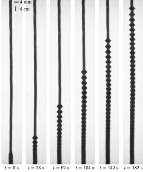
Figure 20: Viscous fluid conduit DSW formation and propagation [184]. Images have a 1:10 horizontal to vertical aspect ratio.
