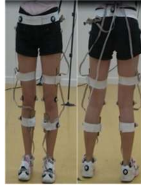
Fig. 5. The attachment of the optical markers and 7 SMUs to the human lower body. The optical markers are placed on the joints to get the position and orientation of each segment to provide ground truth of the fusion results from the measurement of the SMUs.
