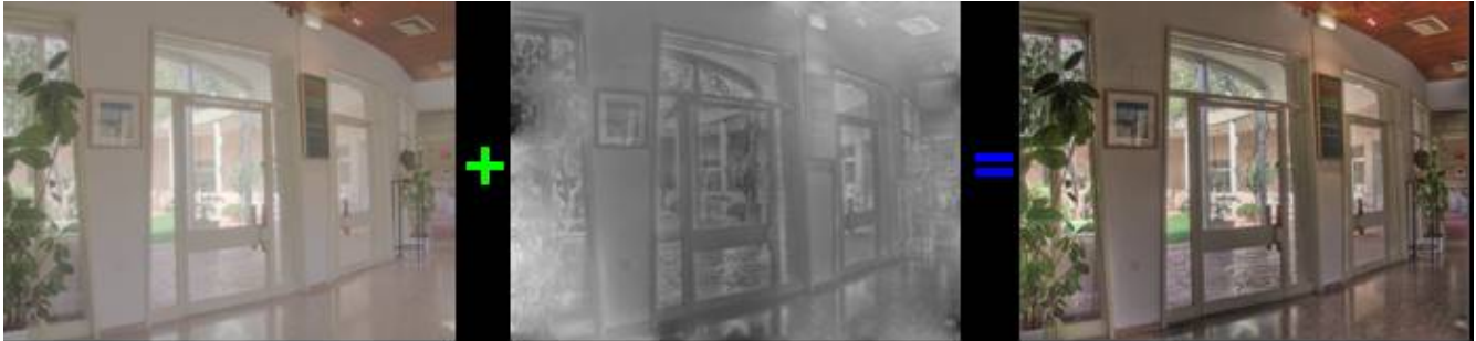
Fig. 1. Direct display of an HDR map in the logarithmic scale (left); the gain map image of the HDR map (middle); the sum of the left and middle images (right). Note the gain map image is only computed for the luminance hence it is shown as grayscale image. Radiance map courtesy of Raanan Fattal, Dani Lischinski and Michael Werman
