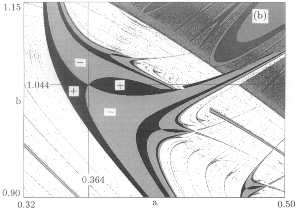
Fig. 4. Magnification of the period-3 shrimp shown in fig. 3, with the lines crossing at a \approx 0.364636 and b \approx 1.044223 indicating the location of the head. (a) Regions of stability, numbers indicating periods; (b) parity of multipliers, eq. (4.2). Heads are unique saddle points inside each cell, dividing them into quadrants .
