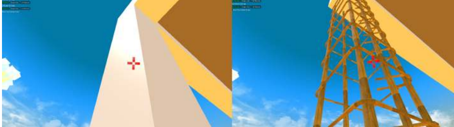
Fig. 3. Concrete column materials being toggled on and off to show the reinforcement elements
