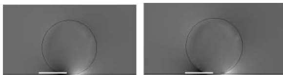
Figure B-1. Map of the pressure distribution for configuration I (left) and configuration II (right). The white line indicates the range of integration of the pressure gradient (see Appendix B for details).
