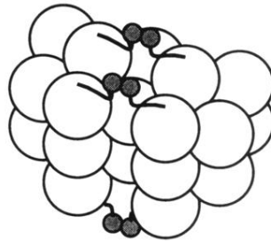
FIG. 1. The geometry of an H_2 molecule along the minimum energy path approaching an Al(110) surface. A molecule approaches the surface in each of the (1 \times 2) unit cells and on each side of the five-layer slab used in the calculation, but the interaction between the molecules is small and does not affect the results.
