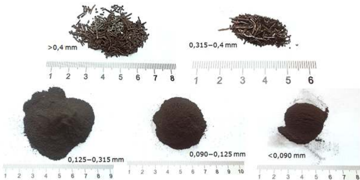
Figure 8. Fractions of pyrolyzed and ground tantalum capacitors
