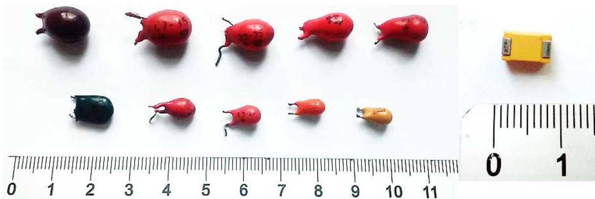
Figure 2. Tantalum capacitor scraps used in this work – LTC (right) and SMDTC (left)
