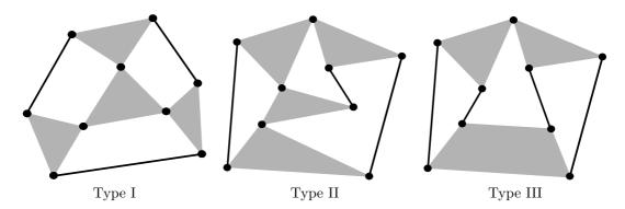
Figure 1: The three three-loop Baranov trusses.
