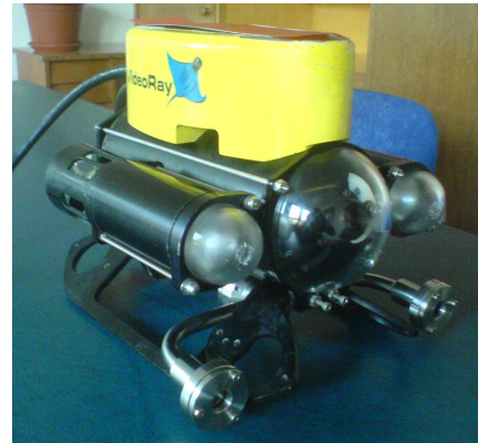
Fig. 1. VideoRay ROV with vision-based distance keeping sensor
