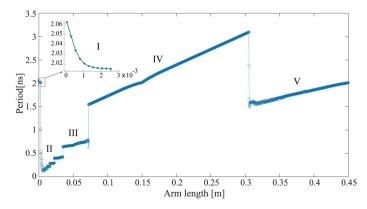
Fig. 2 Switching period as a function of one arm length, while the other arm is 15 cm, for the ring laser regimes (marked I to V) described in this paper
