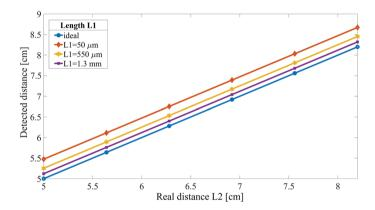
Fig. 6 Distance measured in Regime I as a function of real distance L2 for different values of L1 (ideal: measured distance is real distance)
