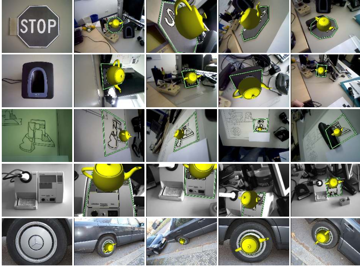
Figure 8. The results of the proposed approach applied to the real world examples. The first image of each row shows the object to be detected and the other images show the detected objects in cluttered images under different perspectives. The estimated pose is visualized using the OpenGL teapot.
