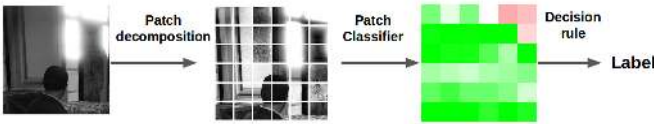
Fig. 1: Pipeline applied to a full-size image: patch decomposition, then patch classification, and finally results aggregation
