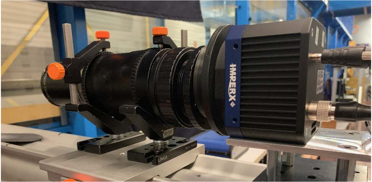
Figure 2: Imaging setup for the present experiment including a 47 MPixel CCD camera and 250mm telephoto lens with extension tube.
