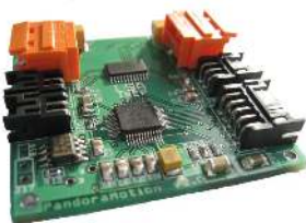
Figure 4. Axis control node DATCOS developed by the ISePorto MSL Team
