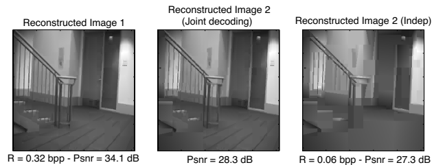
Fig. 4. Distributed stereo encoding of two views. View 1 (left) is encoded at 0.32 bpp and fully transmitted. View 2 (right) is encoded at a lower bit-rate and some of its polynomial coefficients are discarded. Joint decoding of view 2 (center) shows an improvement of the reconstruction quality of about 1dB compared to an independent encoding.
