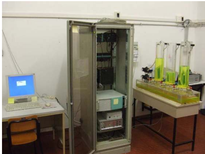
Figure 2.3: The experimental three-tank system.
