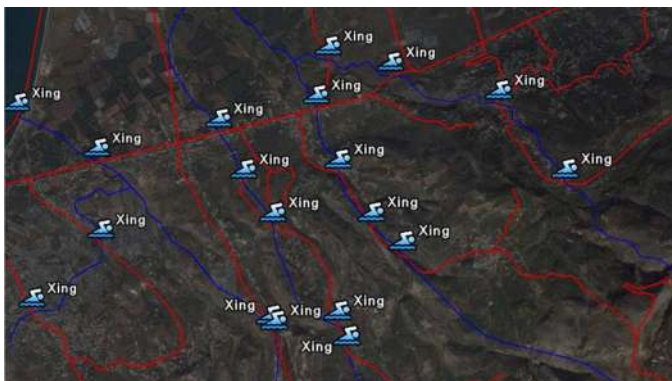
Fig. 7. Example of automatic derived road-water crossings. The geospatial intersection function was applied to the road (red) and river (blue) networks resulting in the highlighted crossings. Satellite image is © Space Imaging International, Ltd., 2005, distributed by European Space Imaging GmbH.
