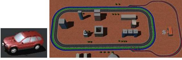
Fig. 5. The vehicle used in the simulations which is equipped with camera, LIDAR, GNSS and radio modules (left). One of the testbeds designed for simulations with more than 1 Km length (right).
