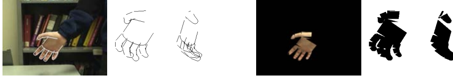
Figure 1: Projected edges (left block) and silhouettes (right block) for a configuration of the 3D structural hand model matching the given image. To aid visualization, the model is also projected following rotations by 35^\circ (center) and 70^\circ (right) about the vertical axis.
