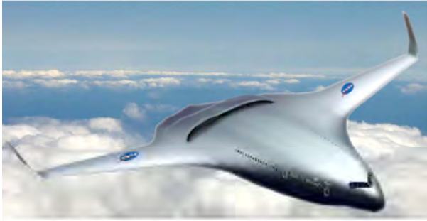
Fig. 11. H3.1 vehicle concept using turboelectric distributed propulsion (TeDP) system by Massachusetts Institute of Technology (MIT) [19].
