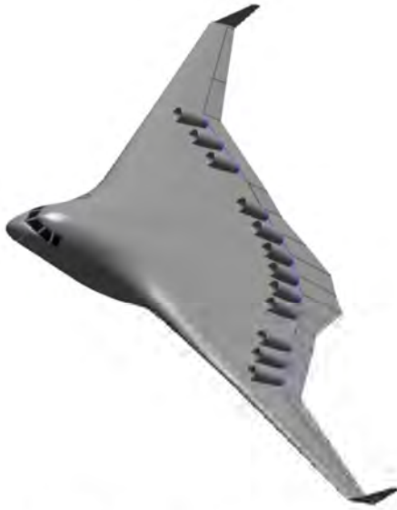
Fig. 4. Cruise Efficient Short Take-Off and Landing (CESTOL) configuration using twelve discrete engines partially embedded in the airframe [6].
