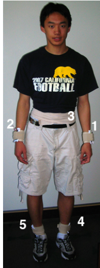
Fig. 1. A subject wearing a body sensor system with the numbering of the sensors superimposed in the image. The sensor system consists of five wireless motion sensors, two on the wrists, one on the waist, and two on the ankles, respectively.
